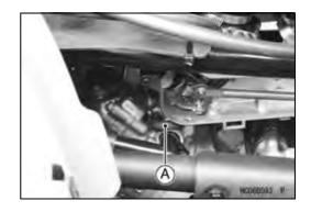
Remove the rear vacuum hose [A] and install the vacuum hose for vacuum gauge.
