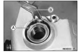
Drive the bearing [A] out using a suitable bearing driver from the bearing driver set.
