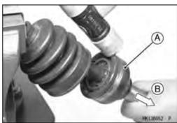
Remove: Circlip [A] Boot [B] Small Band [C]
