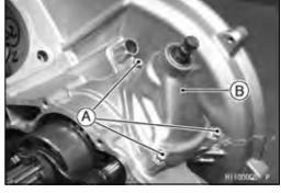
Remove: Shift Shaft Spring Bolt [A] Shift Shaft [B]
