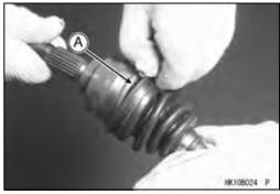
Tighten the large band [A] and bend the tangs securely to hold down the end of the band.
