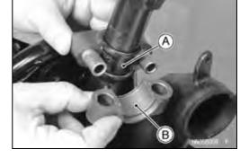
Lubricate the steering stem bearing [A].
