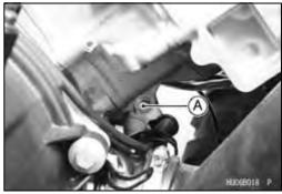
Place a container under the drain plug [A] at the rear cylinder, then remove the drain plug.
