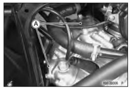
Remove the timing inspection plug [A].
