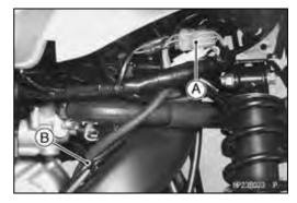
Measure the resistance between the following terminals in the actuator lead connector [A].
