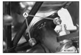
Move the front exhaust pipe rear end [A] under the fuel tank and remove the pipe forward.
