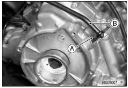
• Turn the crankshaft counterclockwise with a wrench on the alternator rotor bolt until "T-F" mark [A] on the alternator rotor aligns with the notch [B] as shown: the end of the compression stroke in the front cylinder head.
