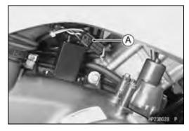
Measure the resistance between the following terminals in the actuator lead connector [A].
