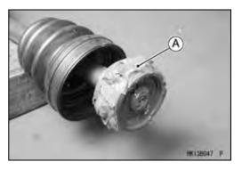
Squeeze about half a tube (30 grams) of the special grease [A] into the bearing cup [B].
