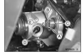
Apply a non-permanent locking agent to the actuator mounting bolts, and tighten them following the tightening sequence [1 ~ 3].
