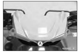
Remove: Handle Cover Screws [A] Handle Cover Front [B]
