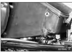
Loosen the clamp screws [A].
