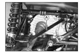
Pull the rear axle [A] in a straight line out of the rear final gear case.
