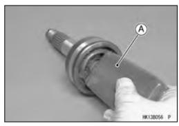
• Tap the shaft end [A] straight with a plastic hammer until it is locked by the circlip.
