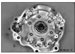
Install: Brake Cam Plate [A]OFit the cam plate and brake camshaft [B] as shown.
