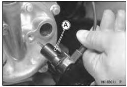
Output Drive Bevel Gear Disassembly
