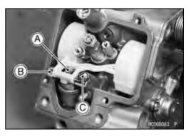
Insert the jet needle [A] into the hole in the center of the vacuum piston [B], and place the spring seat [C] over the needle.
