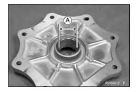
★If the sheave bushing is damaged or worn, replace it.
