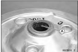
★If the spring is damaged or worn, replace the spring.
