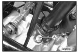
Apply Amoco Rykon Premium Grease No.2 EP (Green): Inside of Steering Clamp [A]
