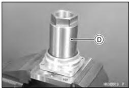
Remove the output driven bevel gear [A] from the output shaft [B] using the bearing puller [C] and spacer [D].
