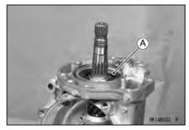
OHold the rear final gear case [A] in a vise, and remove the bearing holder using the socket wrench [B].
