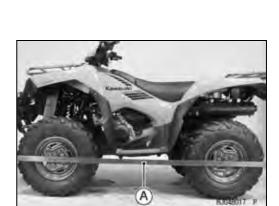
With the handlebar straight ahead, loosen the locknuts [A] [B] and turn the tie-rod [C] until the front wheel on that side is parallel to the straightedge.
