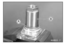
Hold the holder [A] in a vise, and set the output shaft [B] on the holder.
