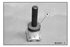
Apply a non-permanent locking agent to the threads of the bearing holder [A] and tighten it so that the deep side [B] faces outward.
