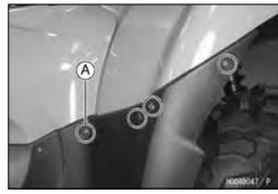
Remove: Screws [A] and Collars Bolts [B] and Collars
