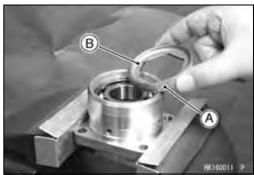
Apply a non-permanent locking agent to the threads of the bevel gear holder nut [A] and tighten it so that the projection side [B] faces outward.
