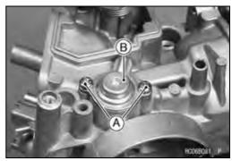
Remove: Diaphragm [A] O-ring [B]
