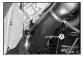
Remove: Joint Duct [A] and Collars
