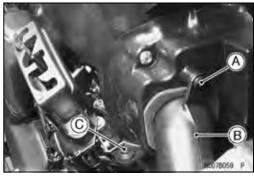
Remove: Air Cleaner Housing Bolt [A]
