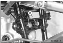
Remove the rear final gear case [A] as shown.
