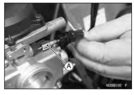
Remove: Screw [A] Holder Plate [B] Starter Plunger
