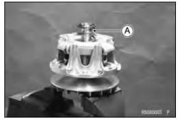
Put the drive pulley wrench [A] on the spider [B] and tighten the bolt [C].
