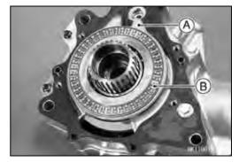
● Check the wear of the disc assembly as follows. ○Measure the thickness of the inner disc [A].
