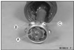
• Apply the special grease [A] to the steel balls and cage.
