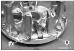
Hold the fixed sheave [A] with the drive pulley holder [B] in a vise.
